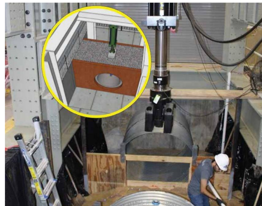
CUIRE soil box test setup for SAPL research project with 330-kip capacity for static and dynamic loads.
