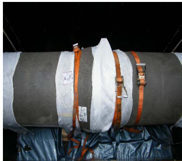
Figure B3. Simulated Damage (Under Fleece)
