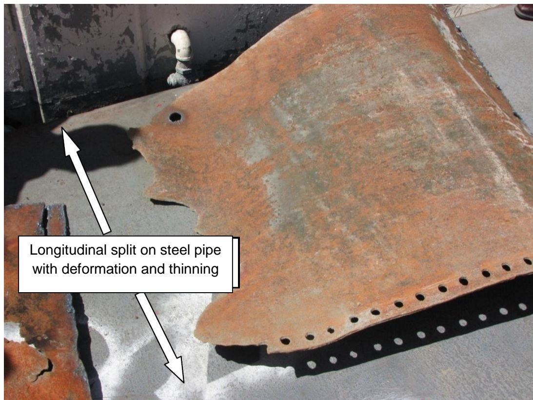
Figure 9.3. Longitudinal Split of Rivet Steel Pipe
