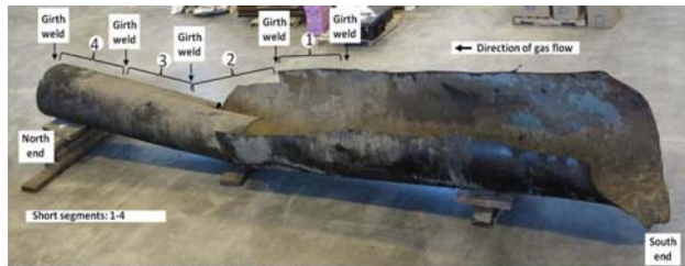
Photograph of the 28-foot-long ruptured section of pipeline
