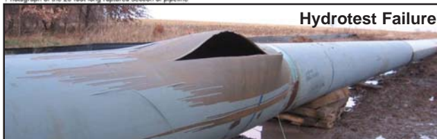
Photograph of the 28-foot-long ruptured section of pipeline
