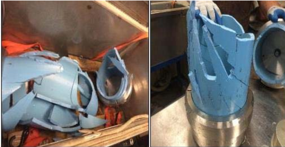
Figure 4.1 Hydrostatic burst test failures (catastrophic) at UTA
