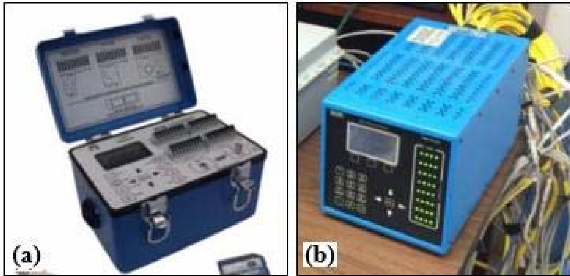
Figure 3.21 (a) P3 data logger for Test 1, (b) System 7000 data logger for Test 2
