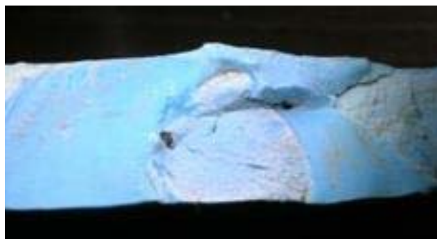
Figure 2.12 Damage from impurities in pipe
