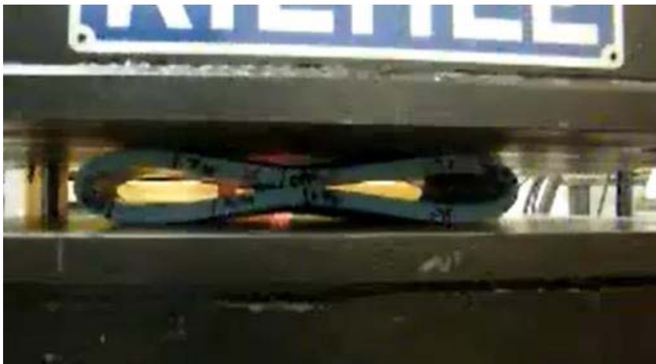
Figure 4.5 Full deflection of iPVC pipe between plates
