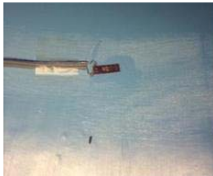
Figure 3.19 Strain gauge attached to iPVC pipe
