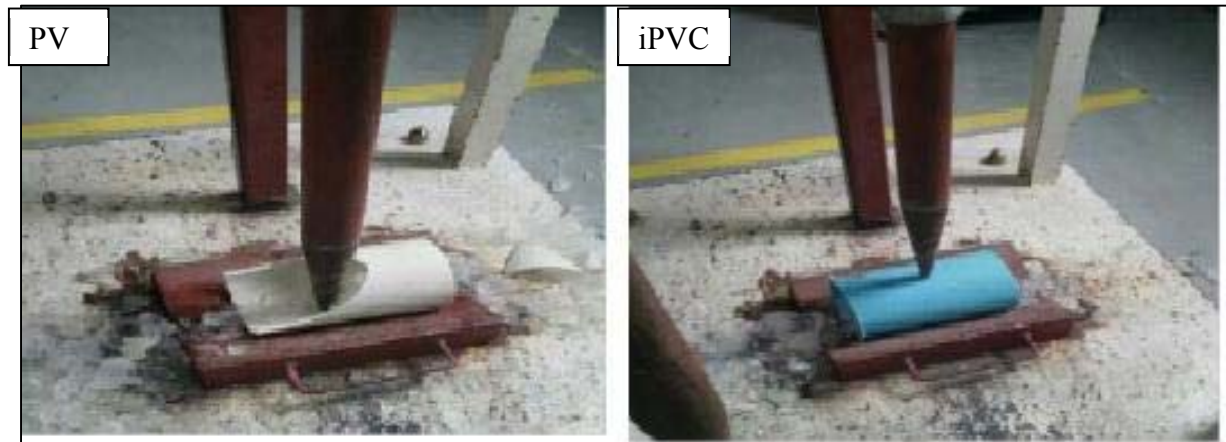
Figure 2.18 Impact testing on PVC pipe on the left and iPVC on the right
