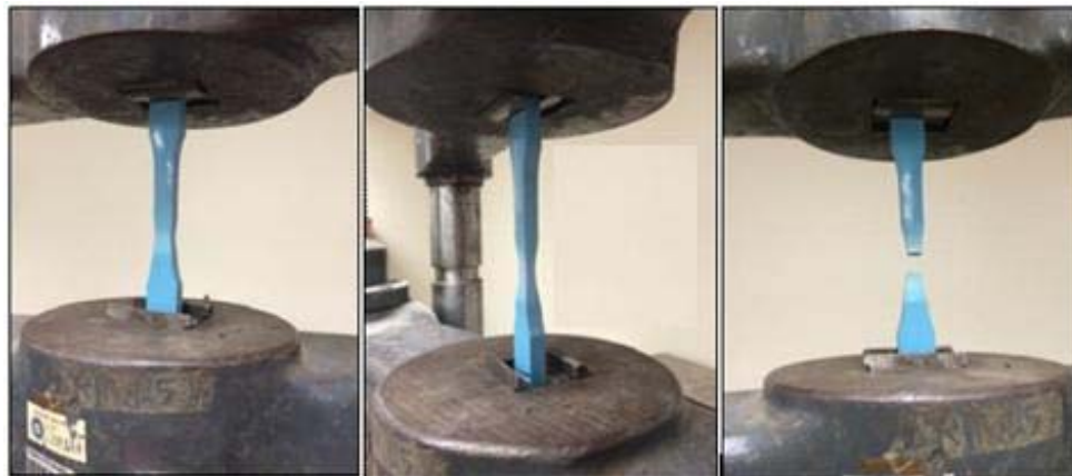
Figure 4.11 Type III tensile testing at UTA
