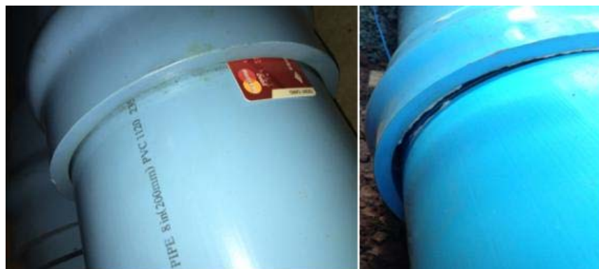
Figure 5.9 Separation at the joint from the new Trelleborg gasket
