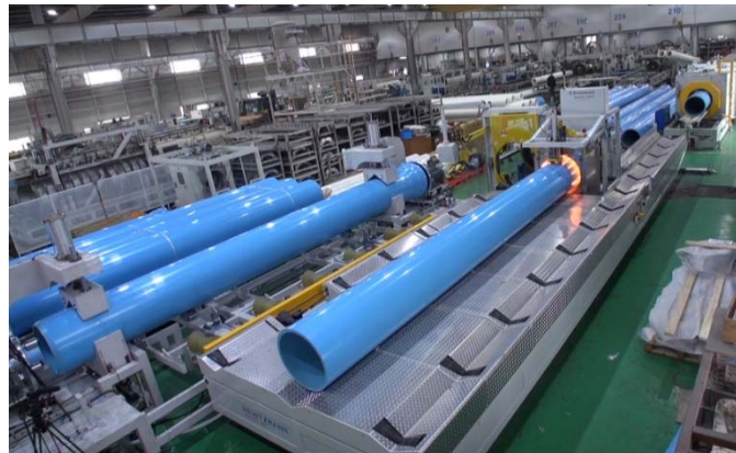
Figure 2.7 PVC extrusion line
