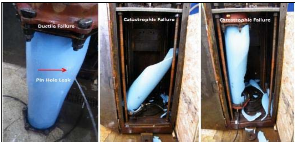
Figure 4.2 Hydrostatic burst test failure (ductile and catastrophic) at Microbac Lab
