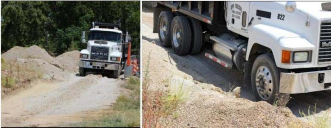
Figure 5.22 Twenty-ton truck creates live load on August 8
