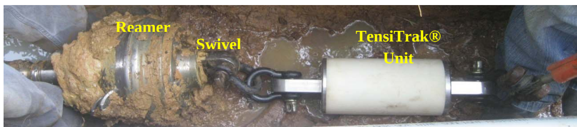
Figure 5-1 TensiTrak® Downhole Assembly
