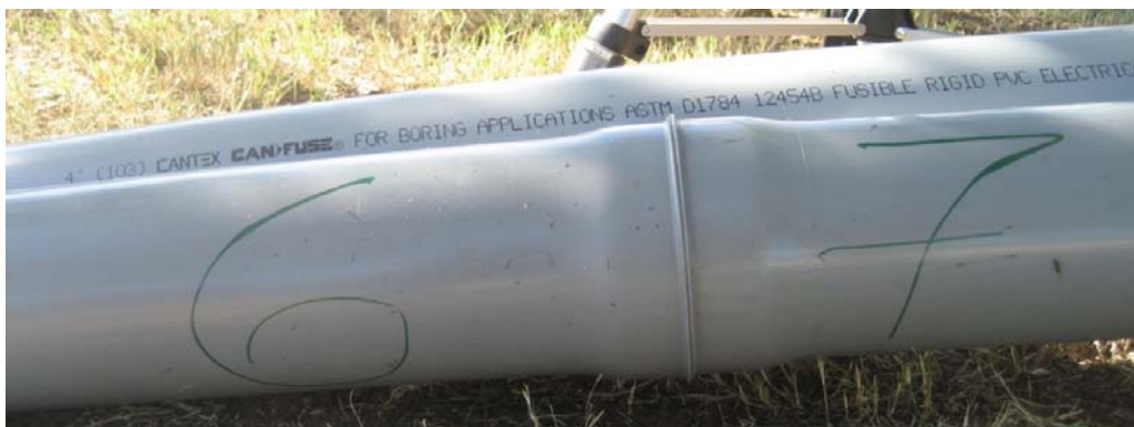
Figure 3-11 Bell Shape End 4-in. (102-mm) Fusible PVC CANTEX Pipe
