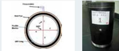
**Figure 5: Long-term Hydrostatic Test Setup**
