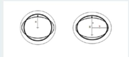
**Figure 6: Liner Deformation under External Pressure.**
